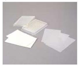
Acetate plate sealers are not gas permeable and mylar plate sealers are gas permeable. All sealers are supplied non-sterile (NS), and they are NOT autoclavable. The dimensions are approximately  $13.3 \times 8.3$  cm.
